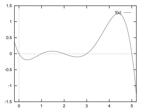
Interpolation polynomial of degree 5 passing through the control points (0,0), (1,0), (2,0), (3,0), (4,1), (5,0):
