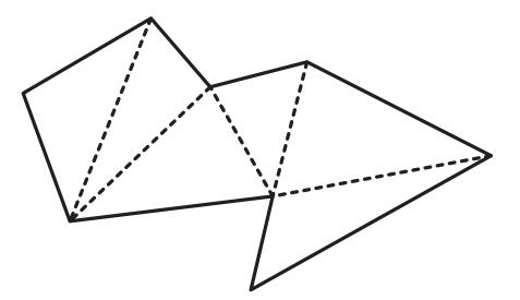
Orientation of polygons: Vertices listed in anticlockwise order to indicate the outside of the surface.
